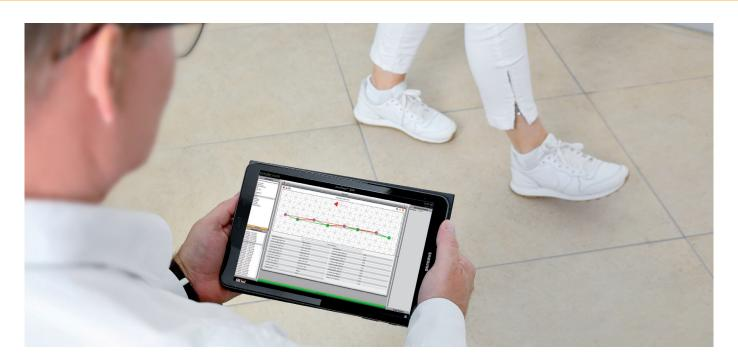
Most gait recording methods are expensive and time-consuming. With SensFloor Gait, neurologists, geriatricians and orthopaedic surgeons can record the gait cost-effectively and, above all, quickly. Because SensFloor Gait is installed underneath the floor, the system is invisible. Patients walk unbiased and naturally over the measuring section.
