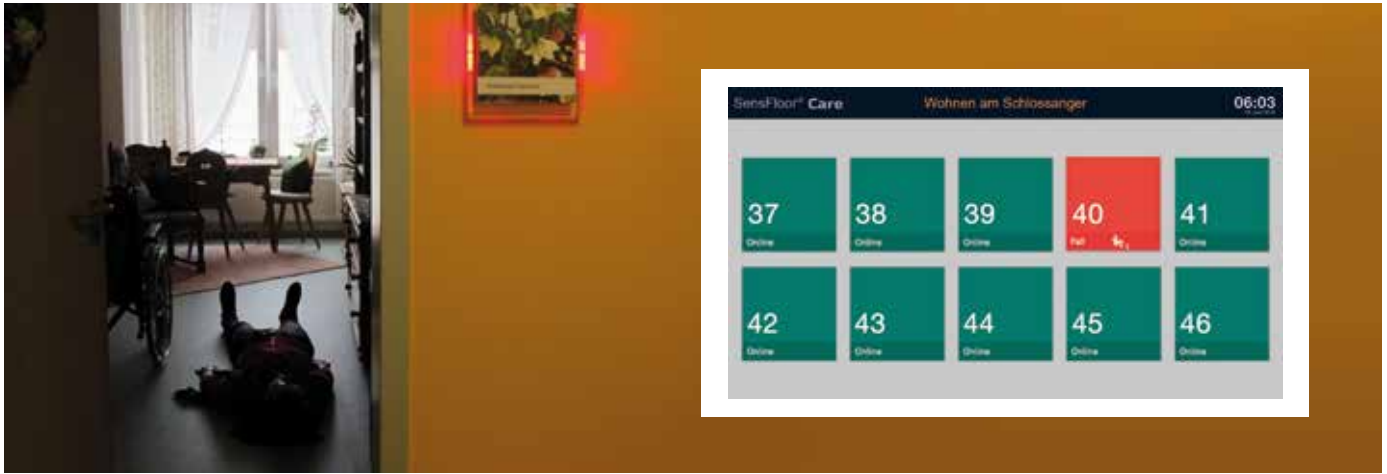
Fall in room 40 – within seconds a member of the nursing staff is in the room
